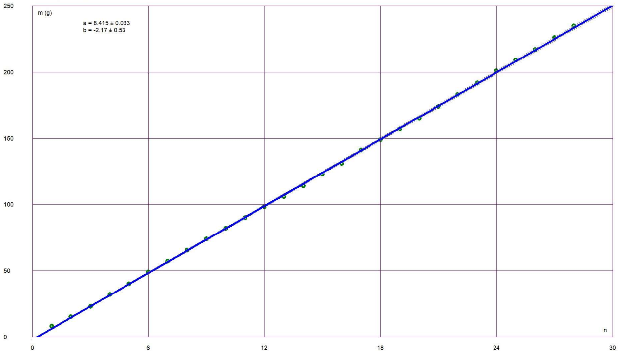
2€ coins with scale (precision 1g) y=ax+b X^2 per d.f.: 0.7978476356 (y), 112.66804 (x) (MDLS)
